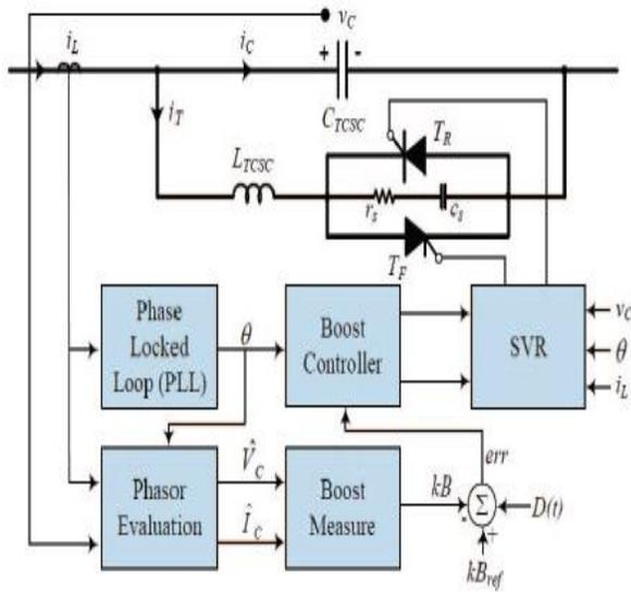
Fig. 3. Block diagram of a TCSC controller.
